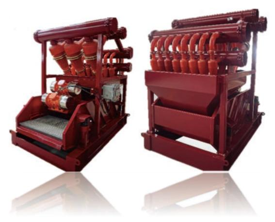
Mud cleaners further process drilling fluid downstream from the shakers. They are engineered to refine slurry through multiple stages of separation by directing flow through the desander (particle size removal to 40  $\mu m$ ) and then the desilter (particle size removal to 20  $\mu m$ ). The discharge from the cones is then screened by the shaker to minimize mud loss.
