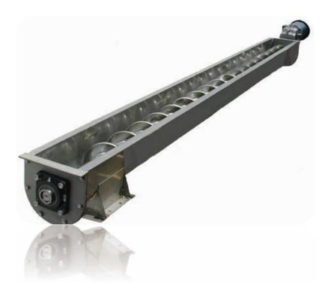
Screw conveyor is designed to delivery drilling cuttings and feed to vertical cuttings dryer or High G dryer for further treatment. Usually, the screw diameter has 3 options : 10 inch, 16 inch, 20 inch; screw length is customer built too, but commonly there are 12~48feet. Furthermore, depends on clients' demand the screw conveyor will be made of different materials. Including carbon steel, stainless steel graded differently.
