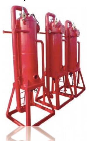
Poor boy degasser is designed for continuous drilling in underbalanced conditions when dramatic pressure surges are normal. In dangerous "kick" conditions, the poor boy degasser allows operators to circulate the drilling fluid by removing large pockets of gas.
