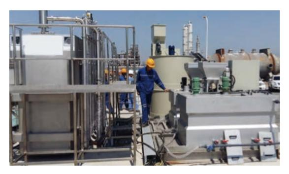
AIPU supply oil sludge treatment system which can recycle oil from oil sludge and dry solids particles with oil content below 2%
