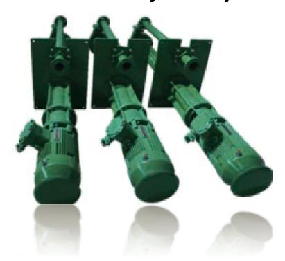
• Submersible Slurry Pump: It is normally used for feeding shale shaker for CBM, HDD or other drilling industry. It is vertical single stage and single suction system and made of abrasion-resistant alloy. The standard length of pump 1.3m but can be customized, the pump is maintenance free and high temperature resistance because no bearing and gland seal between impeller and pump body. Models choose based on required mud flow from 132GPM to 1500GPM.
