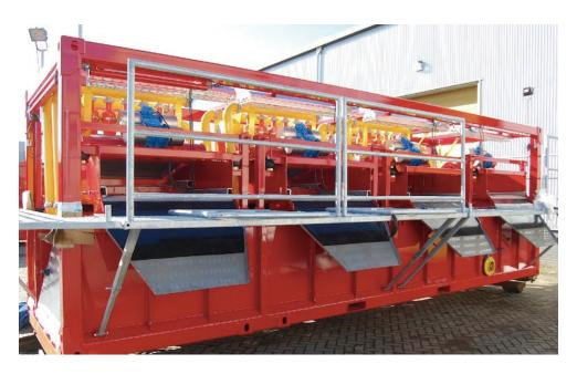
AIPU supply mud recycling system for CBM & HDD & water well drilling and other drilling that need drilling mud, compact design is the key feature for 200GPM / 350GPM / 500GPM / 800GPM / 1500GPM / 200GPM mud flow.
